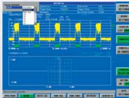
Demodulation of a WLAN(a) signal with the Signal Analyzer R&S® FSQ and option R&S® FS-K91.
